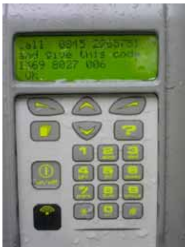
Image: Key buttons in the rental process, such as 'OK' are not marked on the keypad: use depends on the screen.
