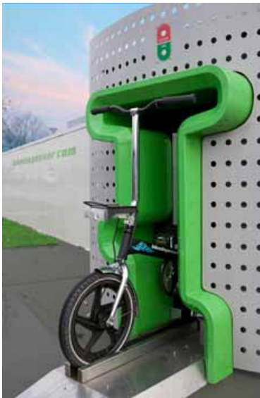
Image: These early Bikedispensers presented smaller bikes, and had different access slots. They were modified to suit the OV-Fiets system.
