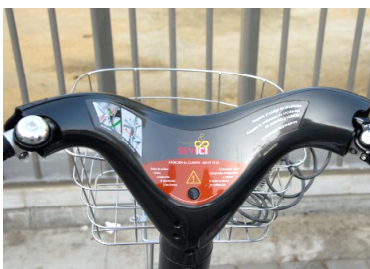
Non-standard handlebars and other components are shrouded in plastic to hide parts which may catch clothing etc.
