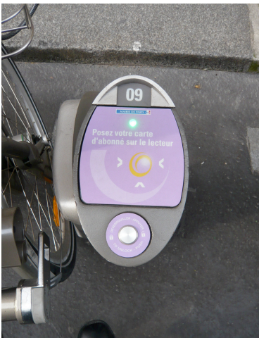
Vélib' docking points allow annual subscribers to swipe their cards directly on the posts to rent bikes
