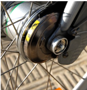
Internal brakes, hub-powered lighting and 'security' wheel nuts and fixing screws.
