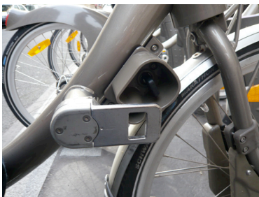
Internal brakes, hub-powered lighting and 'security' wheel nuts and fixing screws.
